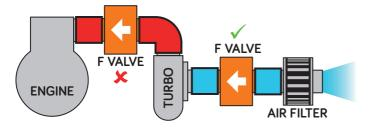
• **Turbocharged Engines with Intercooler:** fit the valve upstream (air filter side) of the turbocharger or downstream of the intercooler. **Do not** fit the valve between turbocharger and intercooler (see schematic below).
