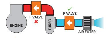
• **Turbocharged Engines with Intercooler:** fit the valve upstream (air filter side) of the turbocharger or downstream of the intercooler. **Do not** fit the valve between turbocharger and intercooler (see schematic below).
