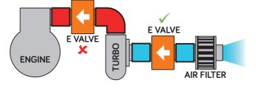
Turbocharged Engines with Intercooler: fit the valve upstream (air filter side) of the turbocharger. If this is not possible the valve may be fitted downstream of the intercooler only if the hose adaptor size for the valve is not too restrictive.
